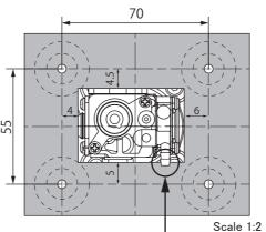
Be careful of contact between the fuel nipple and the firewall. Cracks in the fuel pipe can cause engine malfunction or engine seizure. If the cab body comes into contact with a fire wall, etc., please modify it accordingly.
