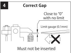
4. Turn the prop by hand to check if the compression is enough. If the gap is less than 0, the valve is always opened sightly and lose compression. Then adjust again.
