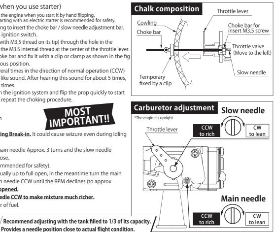
♦ After the initial break-in, keeping the main needle unchanged, open the slow needle Approx. 5 turns CCW from fully closed (Then throttle should be fully closed).
