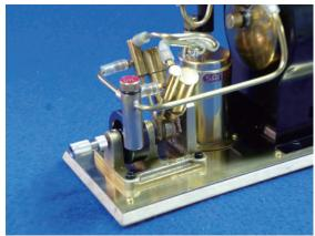
18. Fuel burns out about  $15 \sim 17$ min after ignition, and engine stops naturally. During operation, preserve the notes at the beginning of this instruction, keep stay, pay special attention to fire accident, injury, and breathing combustion gas.
