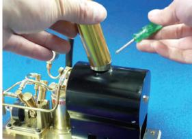
1. Fix the smokestack to the boiler with a fixation screw. Once fixed, it doesn' t need to be removed.
