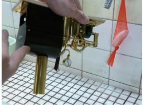
19. After running and it gets cool enough, remove the cap of the safe valve, overflow cap, oiler cap, and drain tank cap, and put the burning tray off. Then have the unit upside down to remove all liquid. (About disposal of the waste liquid, respect local environmental regulations) After that, wipe well the unit body to clean up wet.
