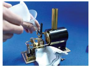
4. Insert the infundibulum deep into the port of safe valve and fill up water, till water comes out from the port of overflow cap. It can be filled about 100cc from vacant. You can cover under the port to wipe out overflowed water. Using pure water is the best bur you can use tap water as long as it's clean. DO NOT use water includes lots of rust or chlorine, or hard water.
