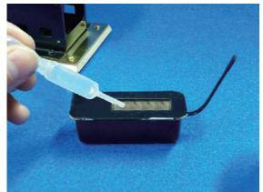
11. Feed the measured amount of alcohol to the burning tray with the dropper. When you spill over the fuel from the tray, wipe out with wet towel well before ignition.
