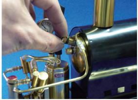
2. Remove the safe valve cap.
