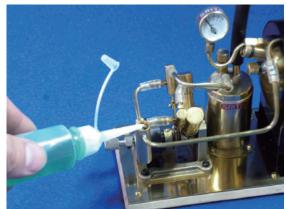
7. Full fill steam oil (blue liquid) up to the oiler and reinstall the oiler cap. Filling any different oil to the oiler causes engine break. It can be coagulated inside the cylinders.
