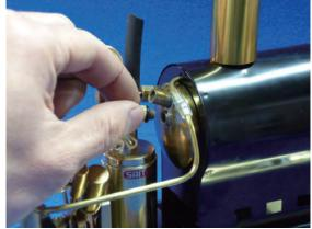
3. Remove the overflow cap as well.
