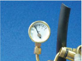
15. When the pressure gauge indicates about 0.5bar, it's ready to start.
