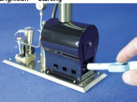
13. For safety, insert the long-nozzle type lighter to the burning tray and ignite. Pay attention as flame comes from alcohol is almost invisible.
