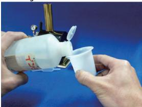
10. Tap the fuel alcohol 20cc with the measuring cup.
