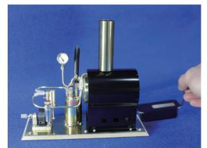
12. After feeding alcohol, set the tray under the boiler and securely insert into the deep. Now it is ready to ignite.
