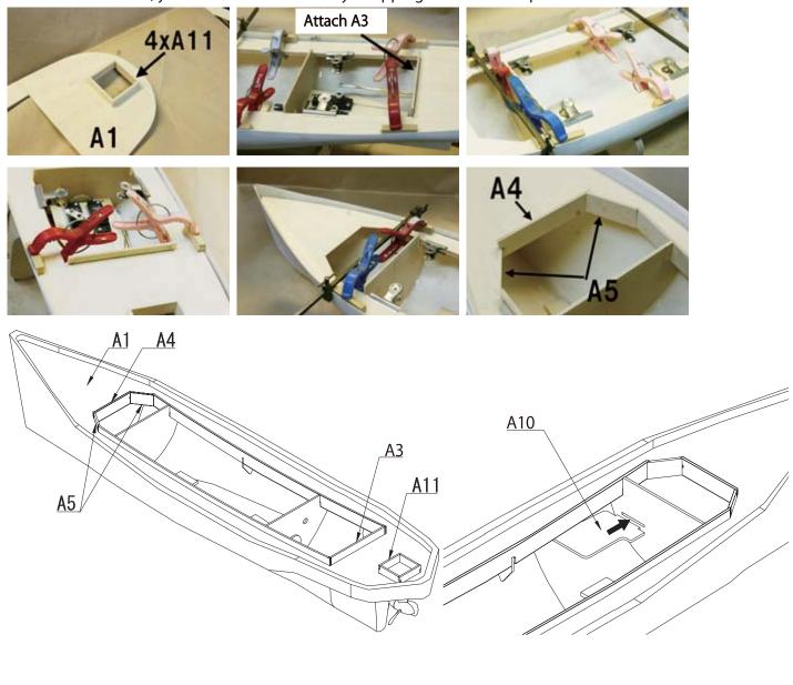
Next, insert step A10 in the rectangular hole in frame plate A6 and attach with "E" so that it is level with A6 and the hull. If it interferes with the hull, attach after filing down A10. A ladder will be attached to A10 later.
