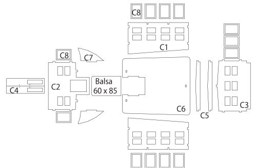
Cut the 2mm thick balsa plate (part no. 61) to a size of 605mm x855mm for the roof-opening portion only. Prepare the plate by rounding the edges. Assemble C1, C2, C3, and C5 by aligning the cut grooves and apply "L" to each attachment point. Cut deck material A (part no. 47) and attach to door C4.
