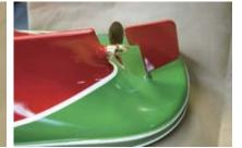
After attaching the rudder A13 to the rudder shaft (part no. 26) with "H", fix with "E" while filling in the gap between the shaft and the rudder
