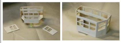
Cut deck material A (part no. 47) to make a door frame and attach to the door. Attach the completed door to the cabin. Attach with "L",
