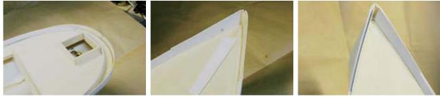
In order to precisely attach to the broadside, place a tie on the straight portions in the same manner as when laying down the deck.
