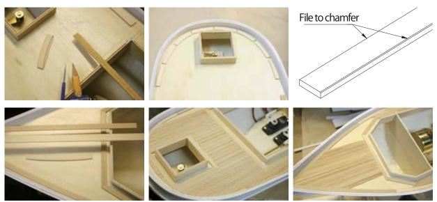
Once you have finished attaching the deck material, before painting, open holes on the port and starboard sides to attach the drain port for deck (part no. 16) from the outside, and attach with "L". Refer to the picture for the location of the drain port for deck (the picture was taken after painting).
