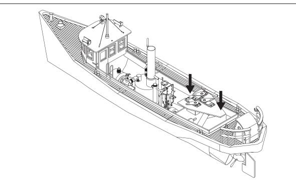
Push in rod S (single end thread) (part no. 38) into the ball joint (part no. 40). Attach the ball joint tip to the servo horn with the screw for ball joint (part no. 41). As shown inthe picture, the portion where one screw was inserted in the rod pipe is to be soldered on after the length is determined.
