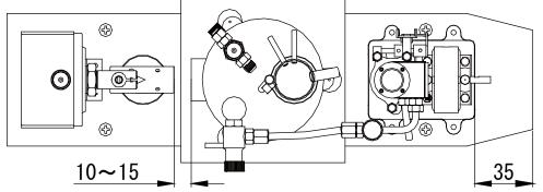
Pass the two pins for the burner stand (part no. 64) through the holes in the burner stand. Leave some play when doing so. Fix the burner by attaching the burner nozzle stabilizer (part no. 62) with the screw for stabilizer (part no. 63) so that it can be inserted in the gap between the nut and the burner unit at the base of the nozzle. Doing so prevents slipping of the burner and from it falling over. It also makes it easier to remove and reinsert the burner when filling it with fuel.
