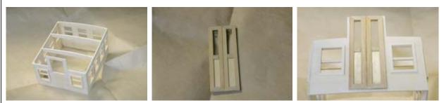
Attach the door to the center of C2 in the assembled cabin with "L". Place roof C6 on top, use a tie and fix with a laundry clip and attach with "E". Once attached, attached C7 with "L". Once C6 and C7 are attached, align the cut balsa plate with the curve of C7, and attach with "L" while fixed with laundry clips. Attach ABS plate A (part no. 49, 2x5) to the bottom of cabin using "L".
