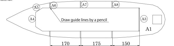
The above is the gap required for the incision on the stringer A2. It may be best to place A2 on the deck to confirm locations and positioning.
