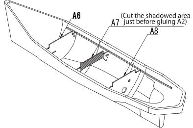
Pass the cypress boards cut to 630mm lengths previously through the grooves on both sides of the frame plate. We call them "b".
