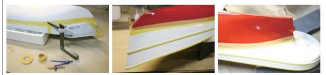
After applying the green paint, removing the masking tape will reveal a distinct white line. This completes the outside of the hull.
