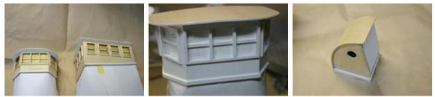
Paint the ABS plate B (part no. 49, 2x5) attached towards the bottom of the cabin and rear box black. Paint the inside of the house as well to make it waterproof.
