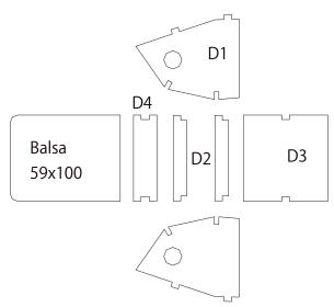
Cut the 2mm thick balsa plate (part no. 61) to a size of 595mm x1005mm for the roof and prepare the plate by rounding the edges. Cut the ABS plate A (part no. 49, 2x5) for the bottom edge so that it can be inserted in the base at the bottom of the deck and attach with "L". Fix the balsa plate with the curve of D1 in the same manner as the balsa roof for the rear cabin, and attach with "L".
