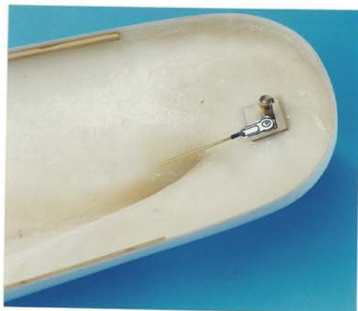
Photo 7 Setting the rudder horn, adjuster, rod and other parts
