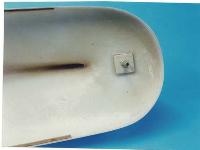
Photo 3 Bonded rudder bearing viewed from the hull inside
