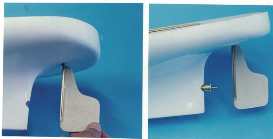
Photo 4 Temporarily assembling the stern tube and rudder
